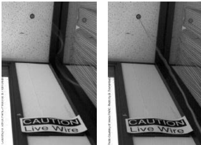
Figure #9-1. “The ‘Dangling String’ is an 8 foot piece of plastic spaghetti that hangs from a small electric motor hanging in the ceiling. . . . A very busy network causes a madly whirling string with a characteristic noise [left]; a quiet network causes only a small twitch every few seconds [right]. Placed in an unused corner of a hallway, the long string is visible and audible from many offices without being obtrusive” (Weiser and Brown, 1995). Courtesy of the Palo Alto Research Center (PARC). Photos by B. Tramontana.
