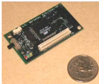
Figure 1: The UC Berkeley mote is a tiny wireless sensor platform for environmental sensing
