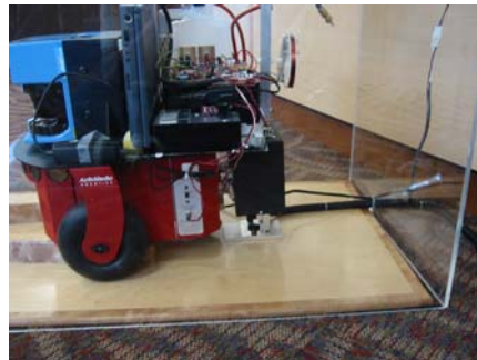
Figure 4: The robot is shown docked in its kitchen cabinet-sized maintenance bay where it can obtain water and recharge
